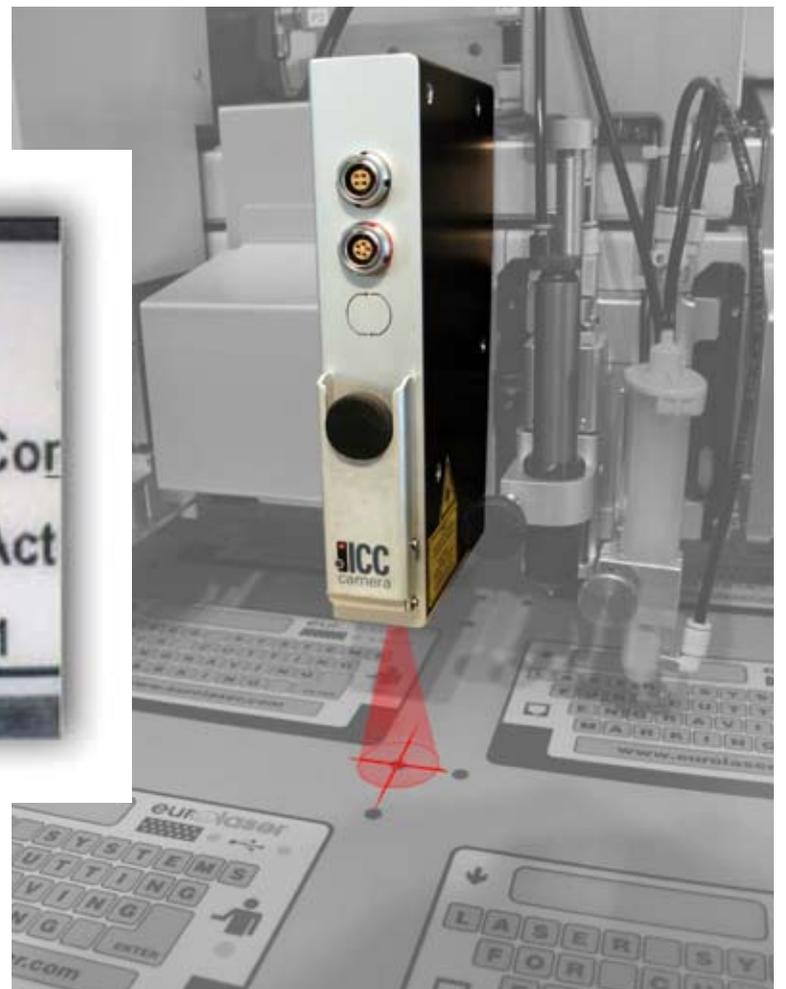
The position of the foil sheet is identified through camera recognition and it is cut precisely
