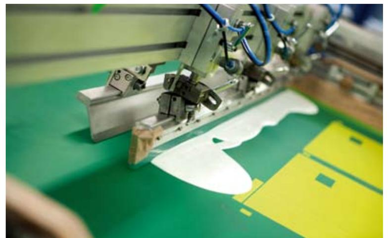
Hybrid process, a combination of digital and screen printing
